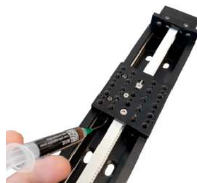
Re-lubricating BLQ linear guide
