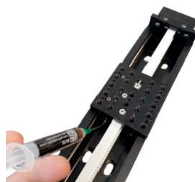
Re-lubricating BLQ linear guide
