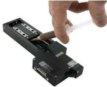
Re-lubricating LRM linear guide
