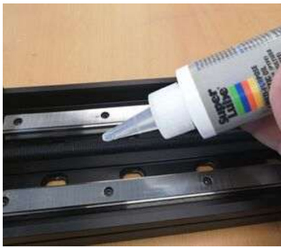
Applying Super Lube to the lead screw
