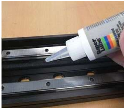
Applying Super Lube to the lead screw
