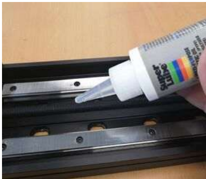
Applying Super Lube to the lead screw
