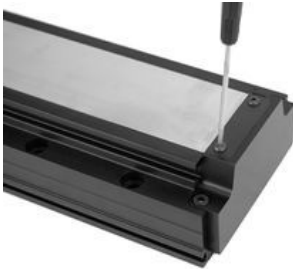
Remove the dust cover clamps at each end of the stage by removing their M3 screws.
