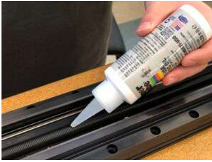
Applying Super Lube to lead screw
