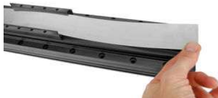
Slide out the dust cover. CAUTION! DUST COVER EDGES ARE SHARP!
