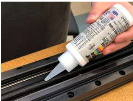
Applying Super Lube to lead screw
