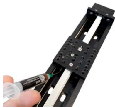
Re-lubricating X-BLQ linear guide
