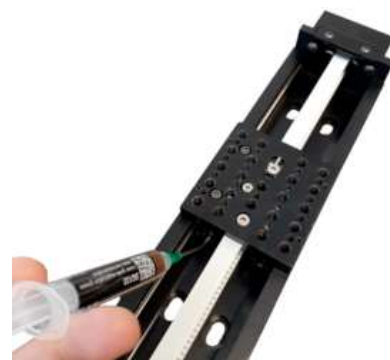
Re-lubricating X-BLQ linear guide
