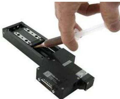
Re-lubricating LRM linear guide
