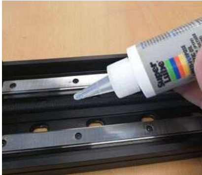
Applying Super Lube to the lead screw
