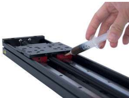
Re-lubricating LRQ linear guide
