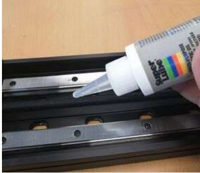
Applying Super Lube to the lead screw
