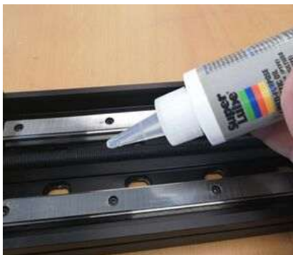
Applying Super Lube to the lead screw
