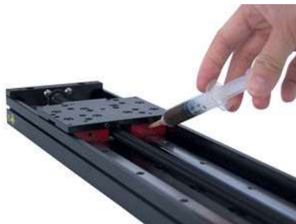
Re-lubricating LRQ linear guide
