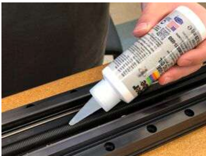
Applying Super Lube to lead screw
