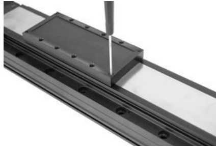
Attach the other carriage end ramp.
