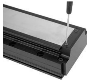
Position the dust cover so it comes close to the clamp holes at each end.
