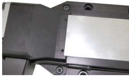
Position the dust cover so it comes close to the clamp holes at each end.
