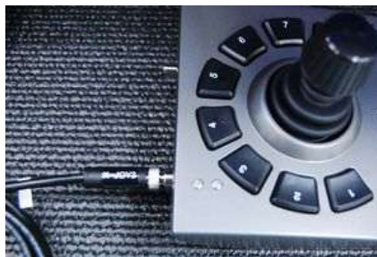
The X-JOY3 is connected to the X-MCC3 through the X-DC06 cable
