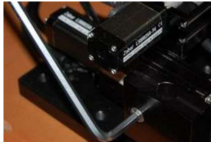
Slide bracket over optical post into desired position and tighten M6 screw with 5 mm allen key to lock M-LSM in position.
