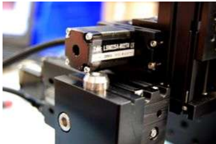
Ensure that the optical post doesn't extend too far, or it will interfere. The above image shows incorrect installation where the optical post will obstruct the movement.
