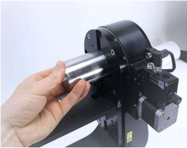
Insert 2" precision alignment pin into the elevation axis stage aperture. You may need to lower the crossmember plate to fully expose the aperture and alternative elevation mount holes.
