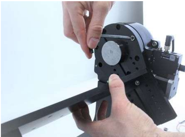
Re-fasten the four M6 screws to re-attach the mount.
