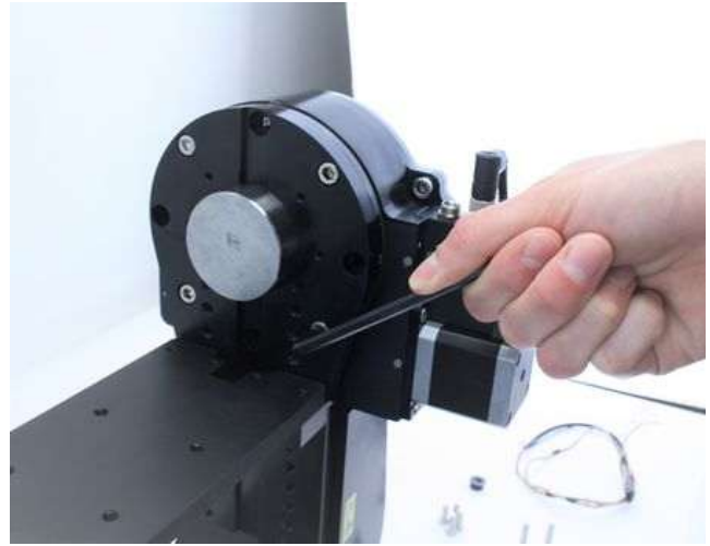
Use a 5 mm hex key to remove the four M6 screws.
