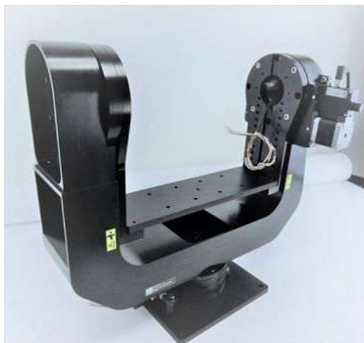
Finished Signal Output Cable Installation.
