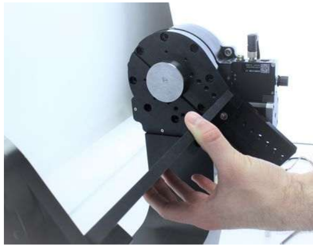
Once all screws are removed, rotate the mount by 45°.
