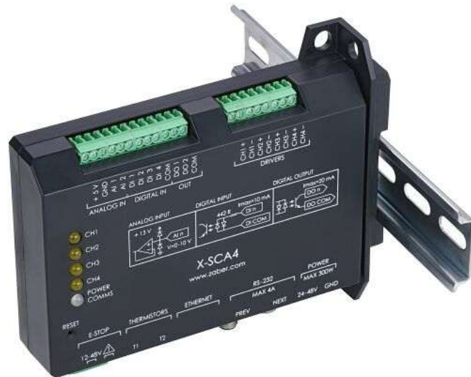
Compact and high density DIN rail mounting with the optional AB258 accessory.
