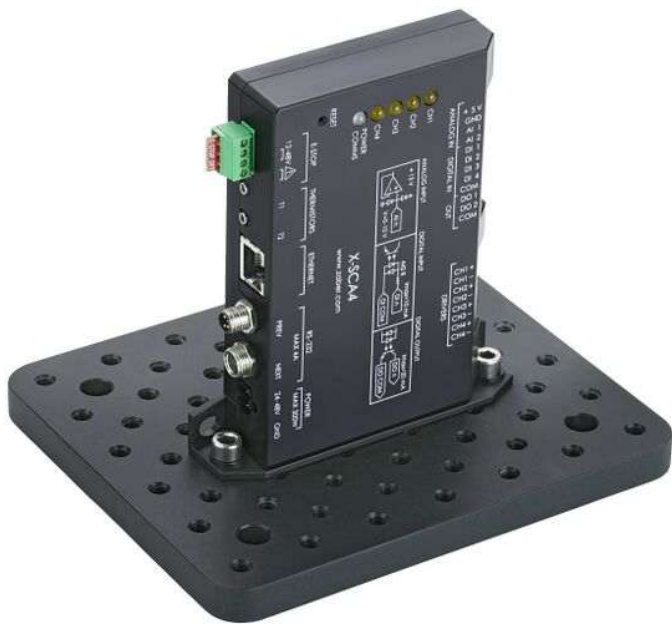
Breadboard mounted controller in the vertical orientation.
